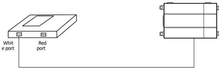
Fig. 7.8 Connecting the communication cable between the controller and the wired water heater controller
